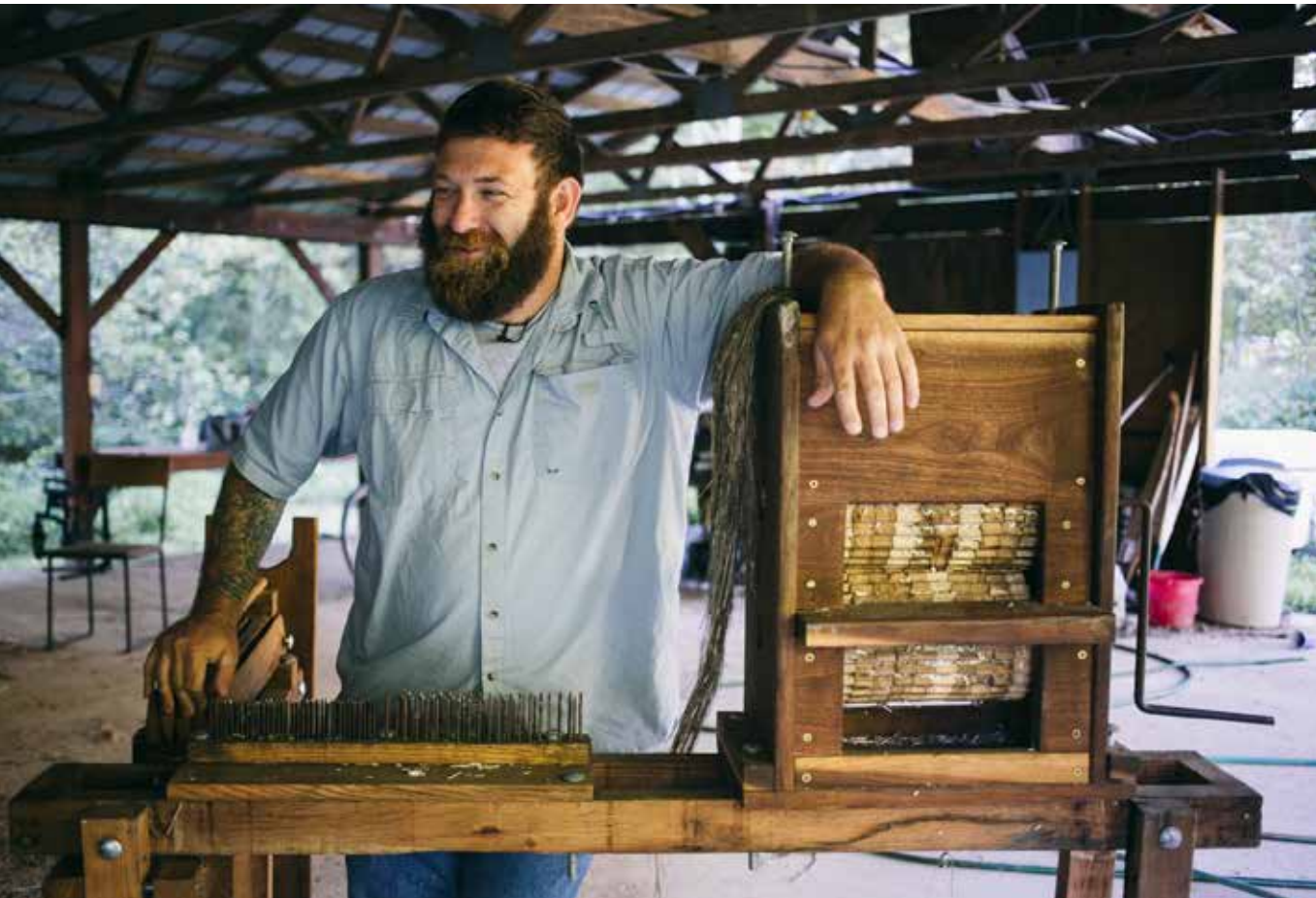
Michael Lewis of Growing Warriors poses with a Decorticator, a hemp-processor built using blueprints patented by Thomas Jefferson. Donnie Hedden
